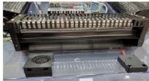
Figure 6. Closeup of the Oion prototype with two plasma ion modules and the tubular fan.
