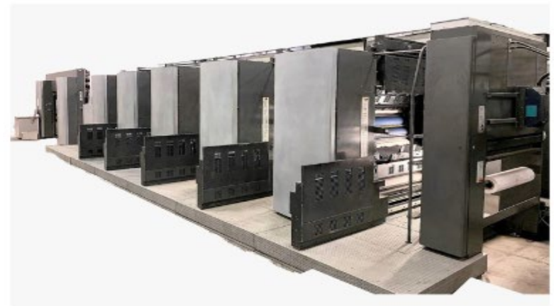
Heidelberg Web M-600 (Web-Fed Offset) 8Color, 40,000 sph(speed)
