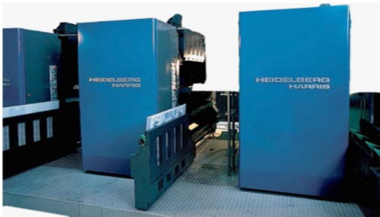
Heidelberg Web M-600 8Color, (Web-Fed Offset) 40,000 sph(speed)
